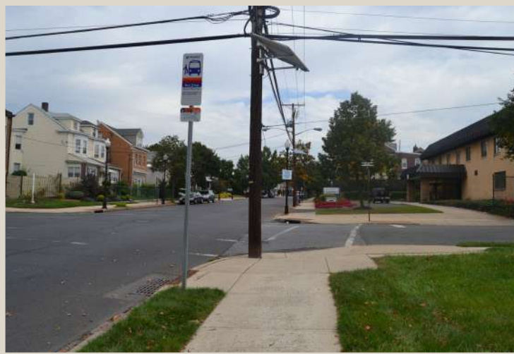
Figure 16. Bus stop with grass strip between sidewalk and curb.
